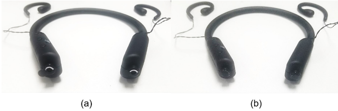
Fig. 14: (a) There is a curved “eyebrows” when the camera is turned on. (b) The camera is completely blocked when the camera is turned off.
